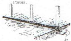
Staple filter materia: to stakes and extend it into the trench.
